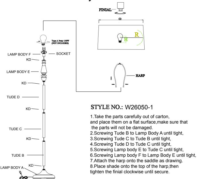
CAUTION: IN ACCORDANCE WITH THE UL REGULATION, THE SHADE SHOULD BE OPEN TOP & OPEN BOTTOM AND "CD" IS BIGGER THAN OR EQUALS TO 4-1/2", "R" IS NOT SMALLER THAN 4-3/4" OR MAY CAUSE FIRE. "H" IS 3\frac{1}{4}".
