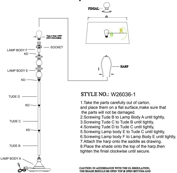
CAUTION: IN ACCORDANCE WITH THE UL REGULATION, THE SHADE SHOULD BE OPEN TOP & OPEN BOTTOM AND "CD" IS BIGGER THAN OR EQUALS TO 4-1/2", "R" IS NOT SMALLER THAN 4-3/4" OR MAY CAUSE FIRE. "H" IS 3\frac{1}{4}".
