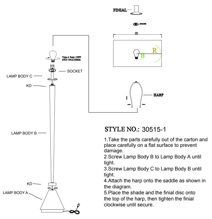
CAUTION: IN ACCORDANCE WITH THE UL REGULATION, THE SHADE SHOULD BE OPEN TOP & OPEN BOTTOM AND "CD" IS BIGGER THAN OR EQUALS TO 4-1/2", "R" IS NOT SMALLER THAN 4-3/4" OR MAY CAUSE FIRE. "H" IS 3\frac{1}{2}".
