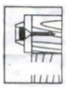
3, Move the furniture into its final position ,taking care to line up the wall bracket as shown in the illustration . Tighten strap until sung .Do not overtighten .
